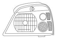
3. Disconnect the electrical connector from the bulb by pulling rearward and unlock the bulb by rotating it counterclockwise.
